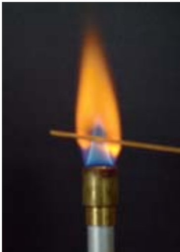
Wood splint soaked in solution of chemical salt.
