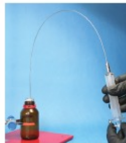
Fig. 9 Removing gas bubbles and returning excess reagent to the Sure/Seal bottle
