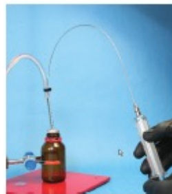
Fig. 8 Filling syringe using nitrogen pressure
