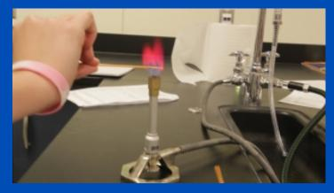
When conducting a flame test, soaking wooden splints in salt solutions and then placing the splints in a Bunsen burner is considered a safer alternative than working directly with flammable liquids, such as methanol, which is not recommended anymore.
