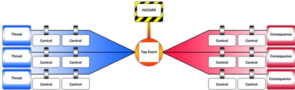
Figure 2. Generic bowtie diagram depicting multiple threats that can lead to the loss of control of a hazard, and intern progress to several negative consequences. 3
