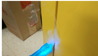
Figure 2. The smoke is pulled through the cabinet door seal. Thus, room air also directly leaks into the cabinet through the door seals.
