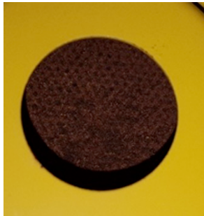
Figure 3. Debris accumulates on the flame arrestor filter that can restrict ventilation flow.
