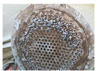
As maintenance workers were scraping the gel out of the heat exchanger when it was opened, it exploded violently, killing 5 of them and injuring 13 others. Subsequent testing of the liquid found in the heat exchanger revealed a composition of chlorosilane polymers containing primarily hexachlorodisilane.
