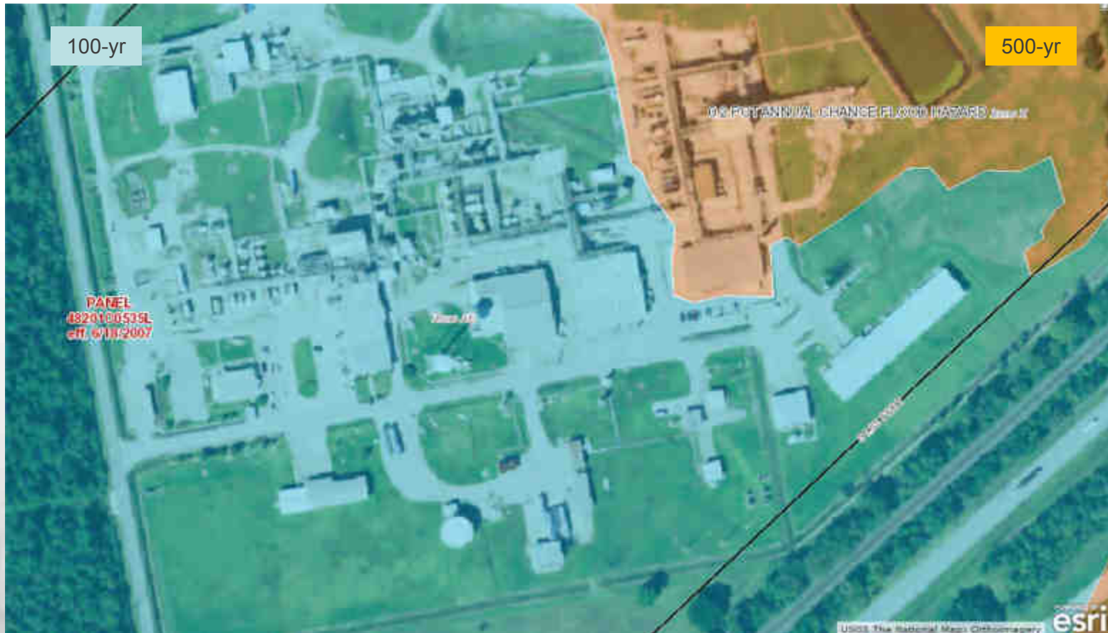
Arkema electric utility supply and organic peroxide low-temperature warehouses now in the 100-year floodplain
