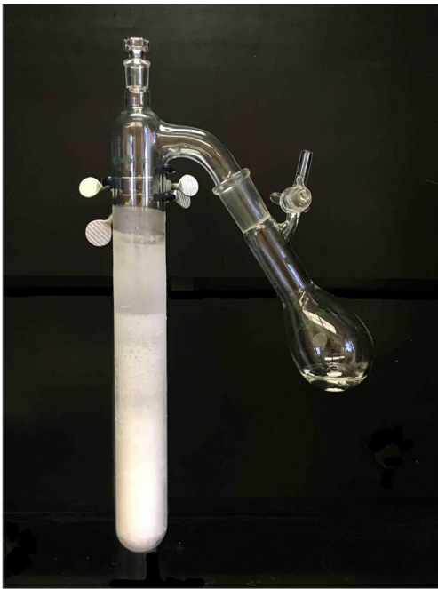
Figure 2. Distillation apparatus with a cylindrical condenser/receiver. The receiver shown is filled with a frozen solvent.
